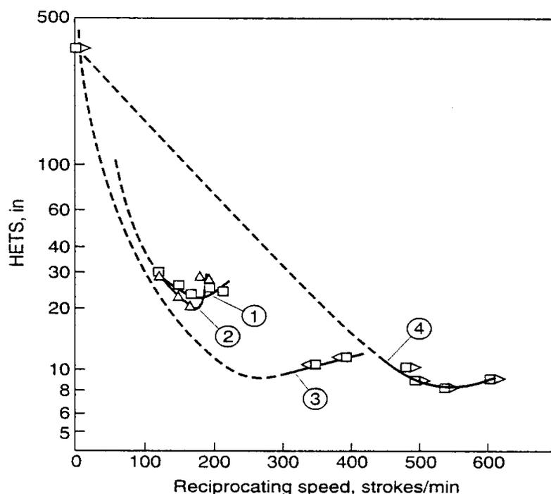
**FIG. 15-51** Effect of reciprocating speed on HETS, *o*-xylene-acetic acid-water system. (Lo and Prochazka in Lo et al., p. 377.)
