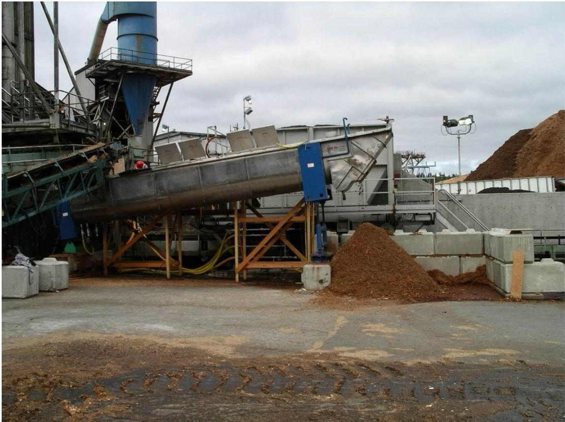
Fig 6 Hog Desalting 5m<sup>3</sup>/hr Pilot Plant
