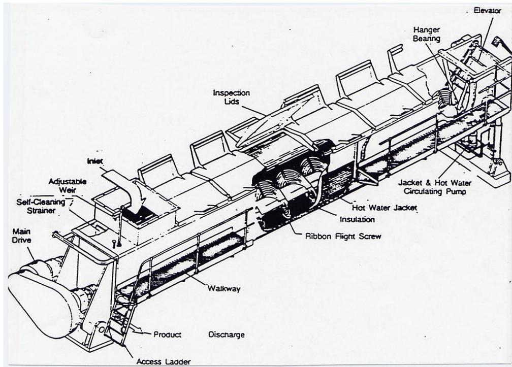
Fig 1 Typical Food Type Counter Current Diffusion Extractor
